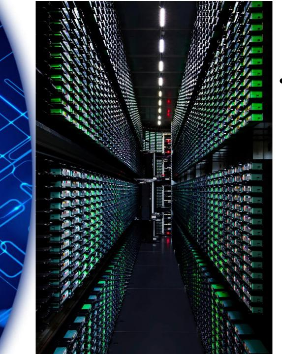
This is the backup center where a robot swaps special cassette tapes that backup the data incase a hardware failure were to occur.
